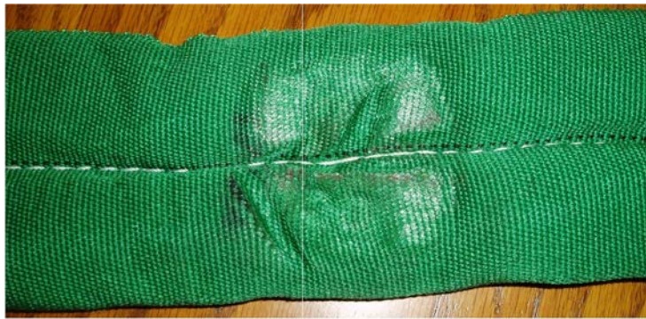
Photograph of the inside end of a sling after cycle testing had been completed
