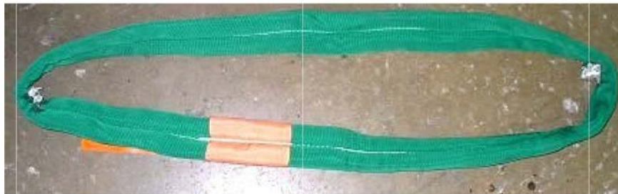
Sling no. 2 after ultimate load testing
