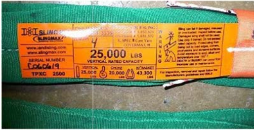
Close-up of tag on slings being tested
