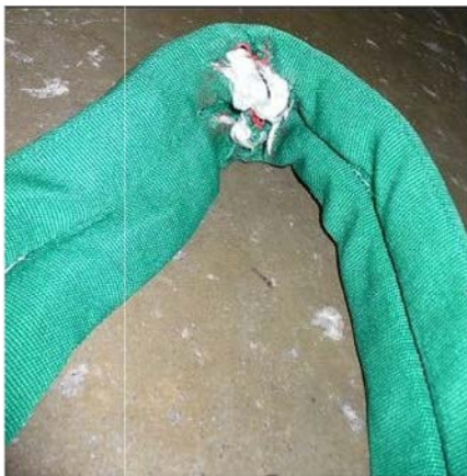
Close up of each end of sling no. 2 after ultimate load testing
