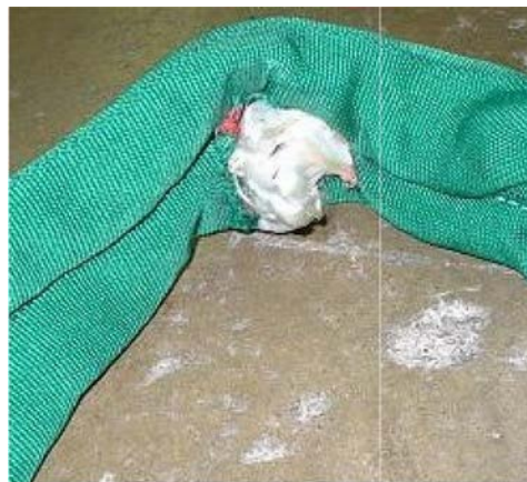
Close up of each end of sling no. 2 after ultimate load testing
