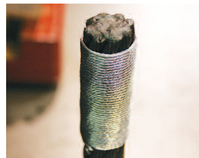
If hose clamps got damaged or are too bulky for the installation you need to replace all 3 of them with a wire seizing.
