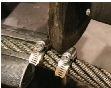
After attaching 3 hose clamps on either side of the cut mark, blade cut the rope.
