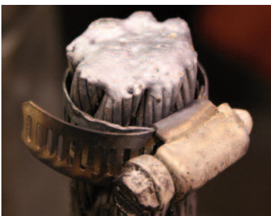
Properly fused wire rope end. If not damaged during the fusing procedure clamps shall be left attached to the rope.
