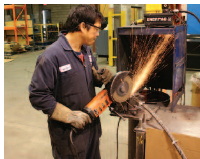
Do not use a grinding wheel but a steel cutting blade; e.g. Elastic # 80EHT230-2.
